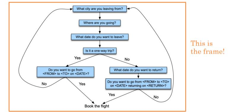
A simple finite-state automaton architecture for frame-based dialog.
