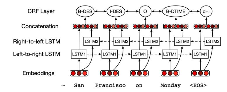
An LSTM architecture for slot filling, mapping the words in the input to a series of IOB tags plus a final state consisting of a domain concatenated with an intent.
