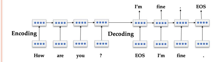
• **Corpus-based method (Seq2Seq):** An encoder decoder model for neural response generation in dialogue. RNN in the above diagram can be replaced with transformer.
